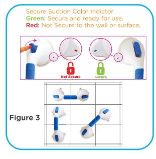
NOTE: Test suction strength by pulling on the handle. If loose, repeat steps 1-3 (see figure 4).
